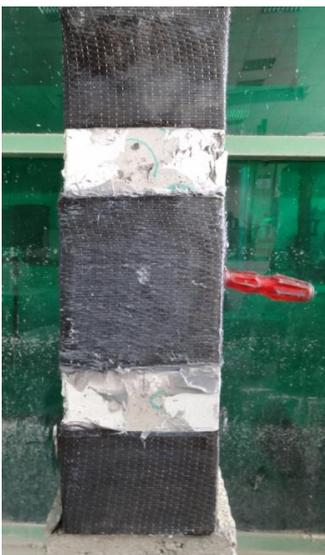
Photo A7–strengthened with pipe and CFRP C7
