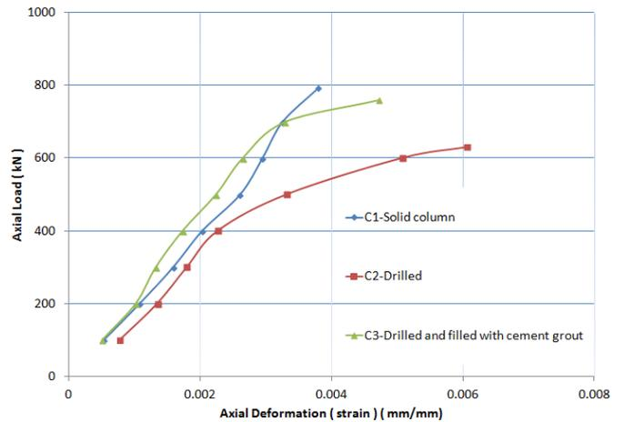
**Fig2. Axial load versus axial deformation for the loaded columns**
