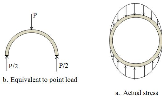
Fig.5- Stress distribution on steel pipe inserted inside concrete
