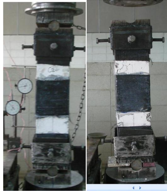
Photo A3 –Strengthened with CFRP,C4
