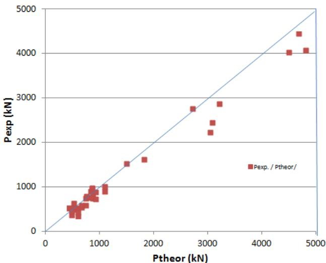
**Fig. 7-Experimental to theoretical carrying capacity of drilled columns ( 37 columns )**
