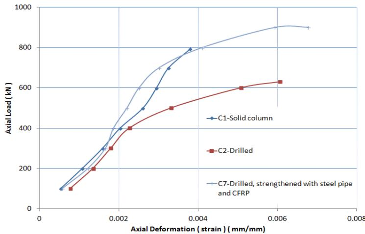
Fig.4 Axial load versus axial deformation for the loaded columns
