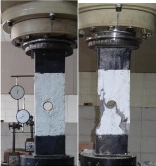
Photo A2 – Drilled Column
