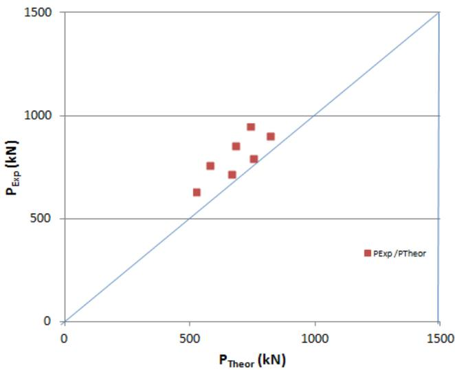
**Fig.6 Experimental to theoretical carrying capacity of drilled and strengthened columns ( from this research )**
