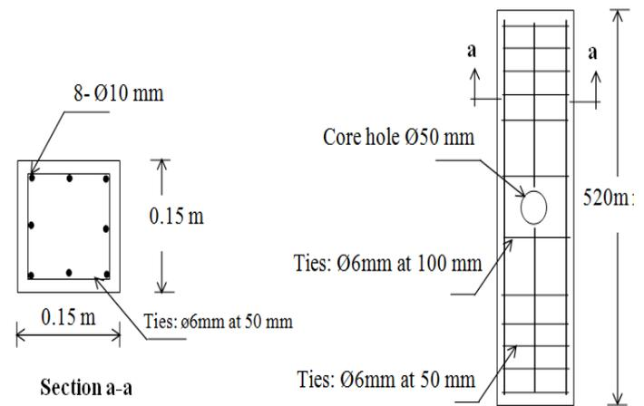
Fig. 1 Details of column reinforcements
