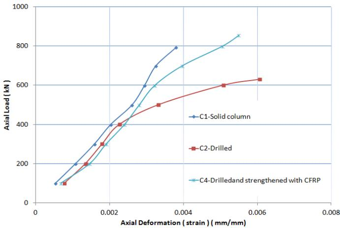
Fig.3 Axial load versus axial deformation for the loaded columns
