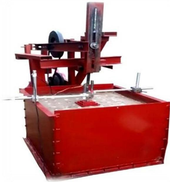
Figure 2: Cyclic plate loading model.
