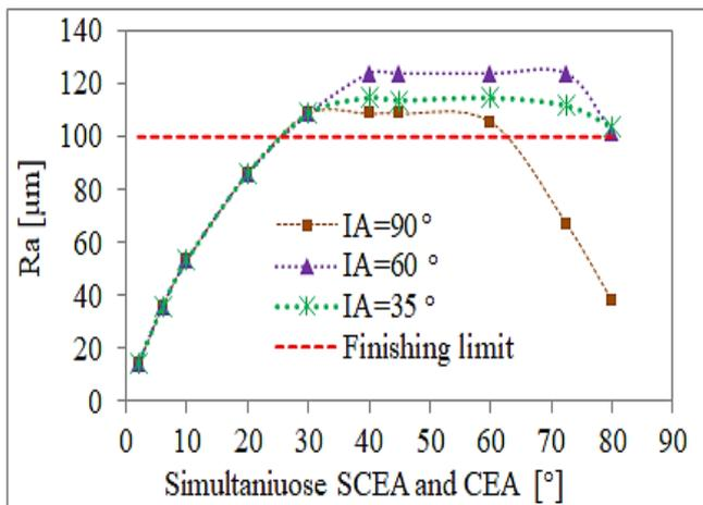
Figure 10: Effect of ECEA with simultaneous CEA on surface roughness by tools of different IA. r = 0.3 mm.
