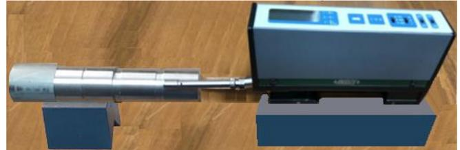
**Figure 3:** The styles type roughness tester during application
